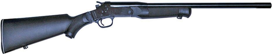
Break open actions are commonly found in Australia in double and single barrel shotguns or air rifles. When the action is open it cannot be fired. The action is usually opened with a release lever located on the top of the action frame. Extraction of cartridges occurs as the action swings open. Some firearms eject the spent cartridges on opening. These firearms have no magazine.
